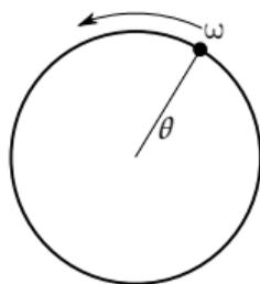
$$\begin{aligned}P_i^{el} &= E_i \sum_{j=1}^N E_j B_{i,j} \sin(\theta_i - \theta_j), \\ I_i &= \sum_{j=1}^N E_j B_{i,j} \cos(\theta_i - \theta_j),\end{aligned}$$
